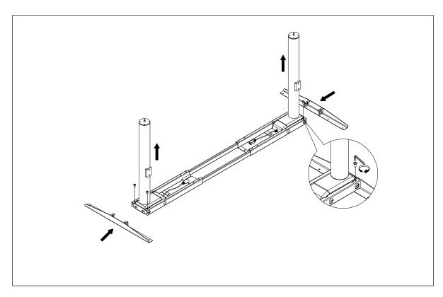
**Step 4** Install the leveling pads
