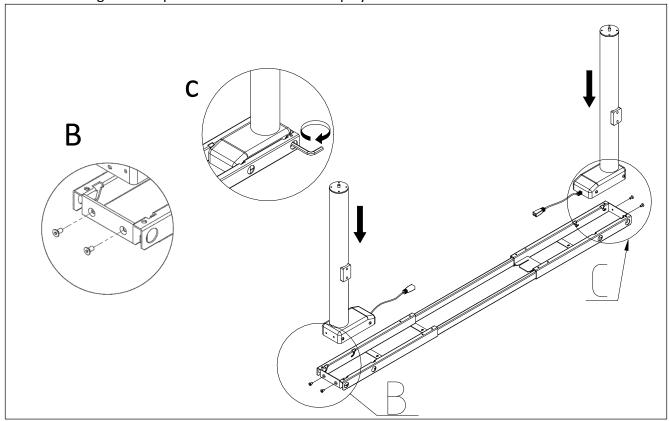
**Step 3**Install the side brackets with Screws 8 pcs M6x16,
