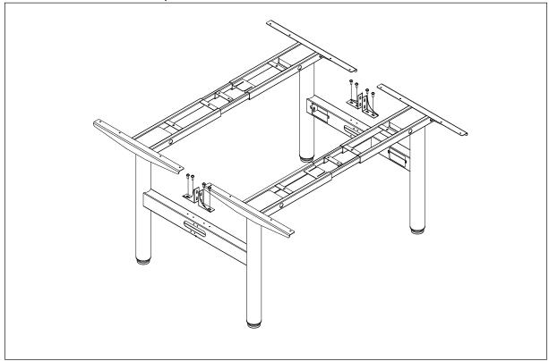
$\label{thm:control} \textbf{Step 7} \\ \textbf{Fix the table top with 26pcs screws ST4x20 ,Install the centre bracket with 4 pcs screws M6x10} \\ \textbf{M6x10} \\ \textbf{M6x10}$
