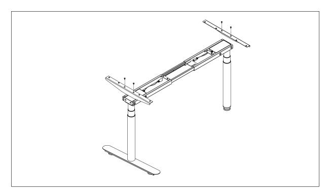
**Step 5**Mount the tabletop and fix it with 14 pcs screws ST4x20; .Fix the centre bracket with 2 pcs screws M6x10; Fix the handset with 2 pcs screws ST4x20
