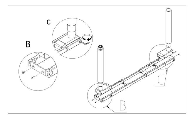
**Step 3**Install the table feet with Screws 4 pcs M6x35, Install the 2 pcs leveling pads
