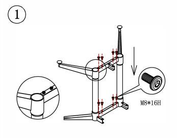
Slide Both The Bottom And Top Cross Bar Into The Left & Right Hand Side End Uprights - Attach Cross Bars With M8 Bolts ( Do Not Completely Tighten Bolts)
