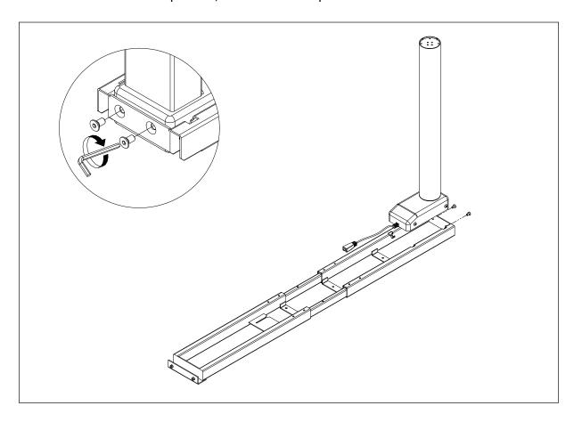
**Step 3**Place the table feet on the column and rotate it and make it align, then tighten the pre-installed bolt.
