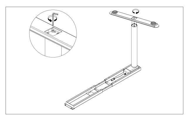
**Step 4**Place the side bracket on the top frame and tighten the bolts.
