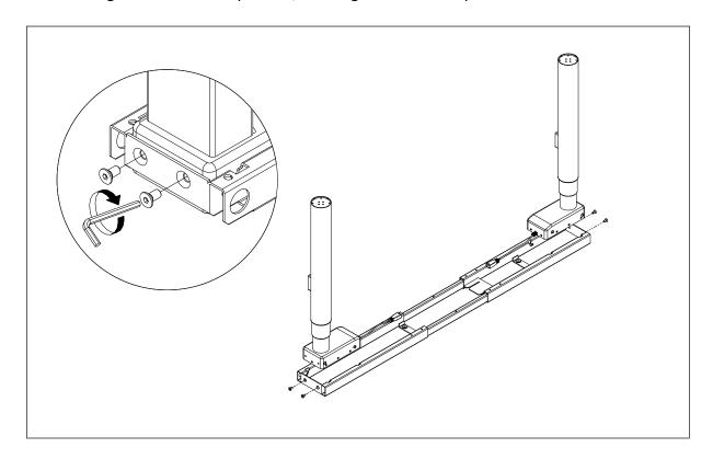
**Step 3**Place the table feet on the lifting column and rotate it and make it align, then tighten the pre-installed bolt.
