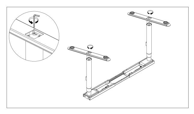
**Step 4** Place the side bracket on the top frame and tighten the bolts.
