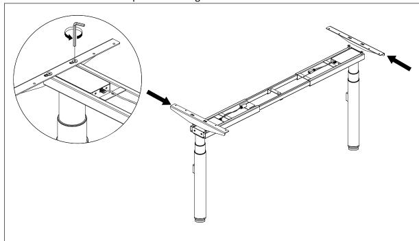
**Step 4**Install the screen brackets with 8 PCS M6x10 Bolts
