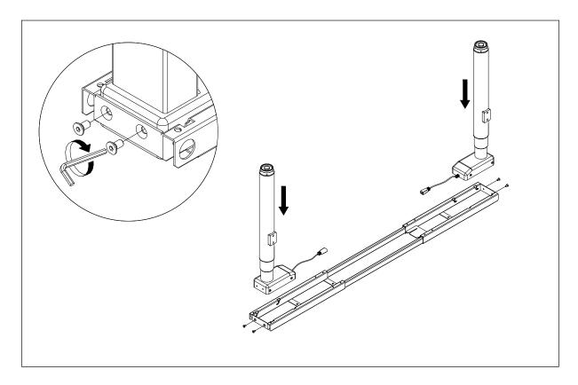
**Step 3** Place the side bracket on the top frame and tighten the bolts.
