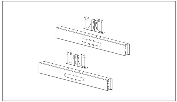
**Step 5**Insert the connected beam and tighten the pre-installed bolts
