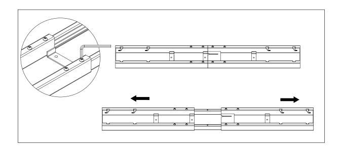
**Step 2**Inset the lifting column to the top frame, fix lifting column with 4pcs screws M6x12 like.
