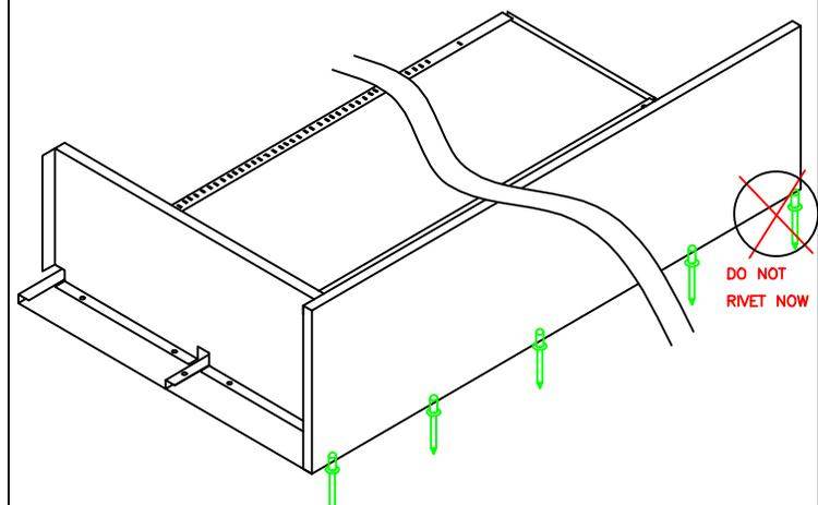
Assemble RH Side with RH back as shown and rivet from outside. **DO NOT** Rivet the topmost rivet which will be riveted along with TOP. Similarly Assemble LH Side.
