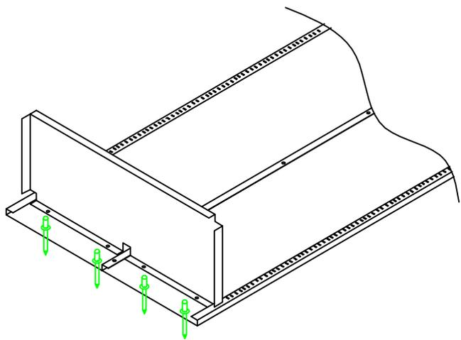
Fix the Bottom tray as shown and Rivet from outside.
