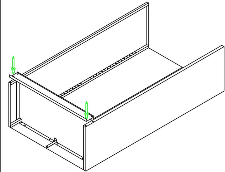
Assemble the Bottom channel as shown and Rivet with sides.
