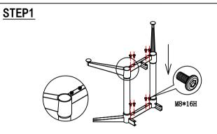
Slide Both The Bottom And Top Cross Bar Into The Left &Right Hand Side End Uprights - Attach Cross Bars WithM8 Bolts ( Do Not Completely Tighten Bolts )
