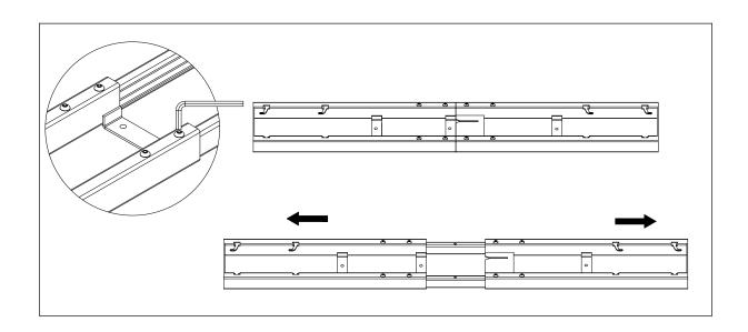
**Step 2**Inset the Column to the top frame, fix lifting column with 4pcs screws M6x12 like.
