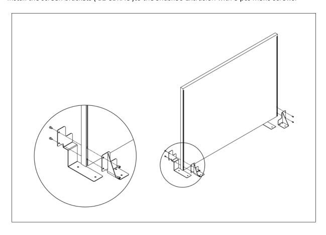
**Step 3**- Fix the screen brackets (B2-SBRAC) to the desk frame with 10 pcs M6x10 screws.
