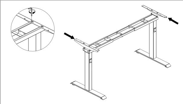
Step 5 Mount the tabletop and fix it with 14 pcs screws ST4x20;
