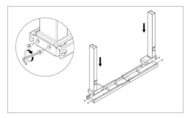
**Step 3**Place the table feet on the Column and rotate it and make it align, then tighten the pre-installed bolt.
