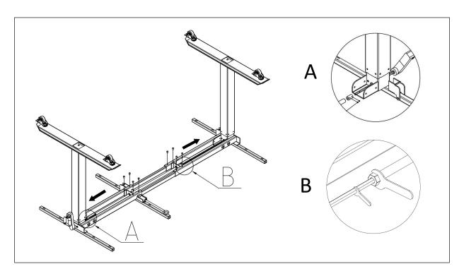
**Step 6**Stick the rubber pads on the top frame before table top mounted, fixed with ST4x20 Screws.
