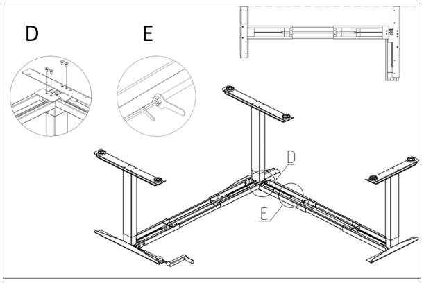
**Step 6**Fix the desk frame to the tabletop with 17 PCS ST4X16 screws
