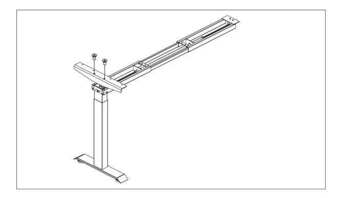
**Step 5**Connect the return frame to the single desk and fix it with 2 PCS M6x12 Bolts
