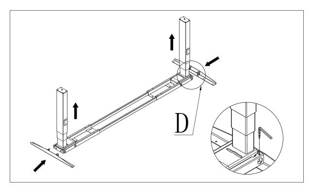
**Step 4** Install the leveling pads
